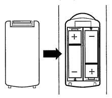
To avoid damage from possible battery leakage, remove dead batteries or batteries that will not be used for a long time. For replacement use type R3 or AAA batteries.
